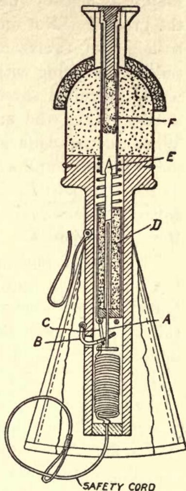
FIG. 5. A German parachute grenade
