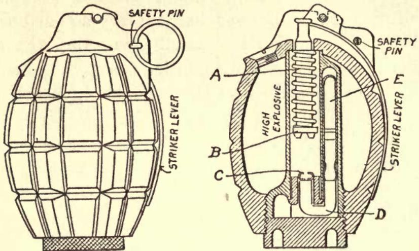
FIG. 4. Details of the Mills hand grenade
